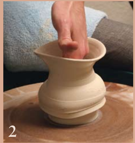
2 Stretch the form from the inside until it is near the point of collapse.
