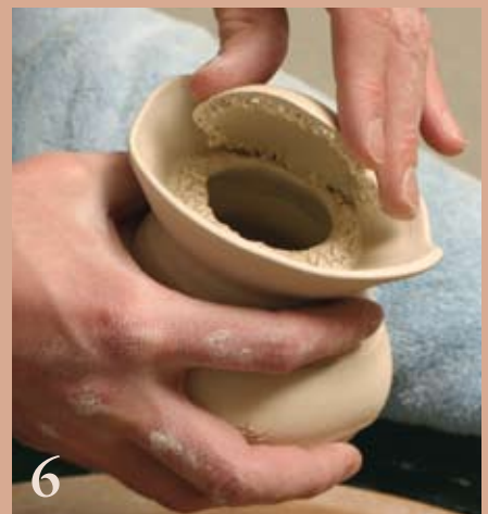
6 Stretch a slab top into a shallow bowl shape and add it to the flange.
