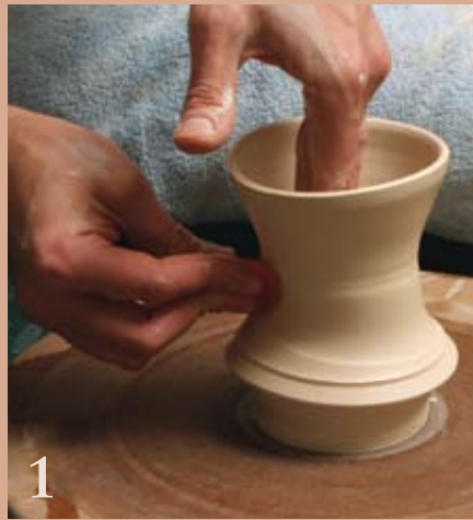
1 Compress and smooth the cylinder then make a spiral on the bottom half.
