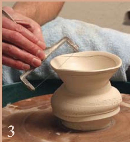
3 Cut the rim with an up-and-down motion using a cheese slicer.
