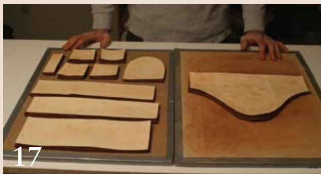
17 Cut all the pieces for building the cabinet using the templates before assembly begins.
