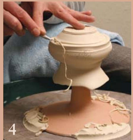
4 Small trimming tools help create crisp, clean lines and transitions.
