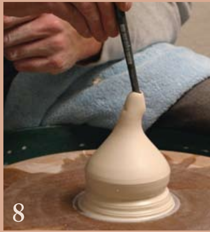
8 Stretch the back of the spout using a blunt tool.
