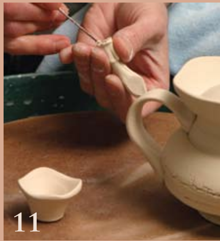
11 Score the knob and the inside bottom of the stopper then attach.
